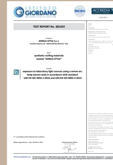
Test report 3.000 h of Xe-arc WOM, UNI EN ISO 4892 + 9.500 h of Q UV-A, test ASTM D4329 - Cycle A
